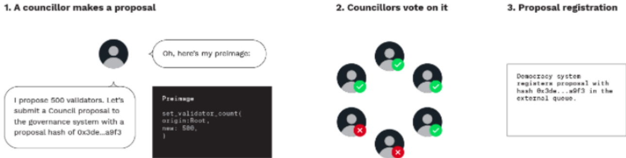
Figure 11: Demonstration of the acceptance of a proposal through a unanimous group decision amounts council members [86]
